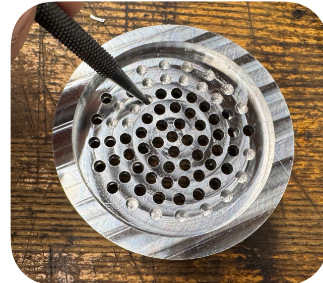
Filed 0.003" in z to clear out holes
