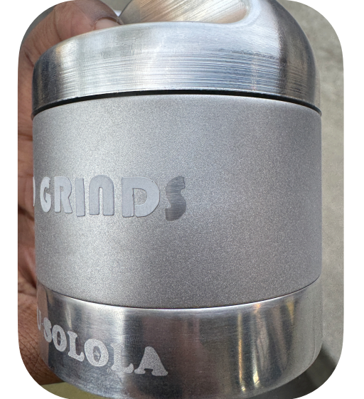
Bead blasted Enclosure to create contrasting finish. Handle was left with machine finish
