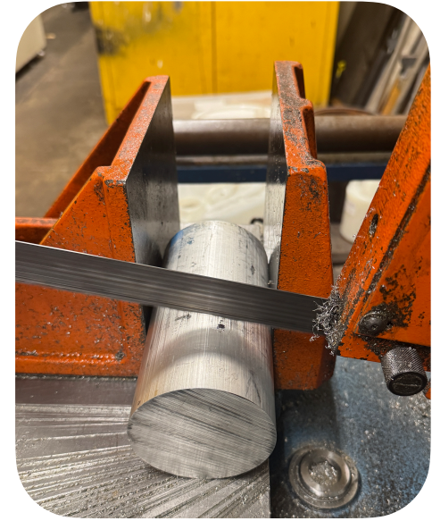
Rough stock cut with horizontal bandsaw
